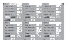
The 9" Touch Screen Computer provides real time display of process variable, set point, load current, load demand (%), operation mode type, alarm status and alarm type for any 6 circuits at a time as well as alarm status for all other circuits.
